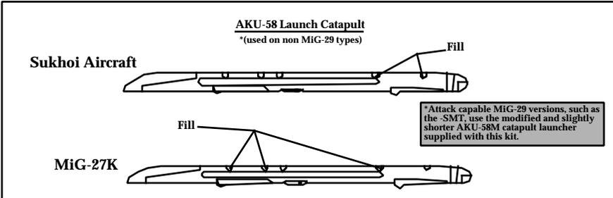
\*Attack capable MiG-29 versions, such as the -SMT, use the modified and slightly shorter AKU-58M catapult launcher supplied with this kit.
